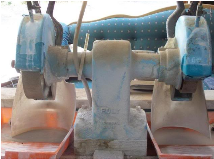
This is the work horse. 10" Poly arbor (very hard to find) with 8" 50 grit wheel and 6" 180 grit wheel.
