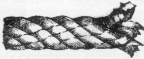
Three strand twisted or laid rope.
